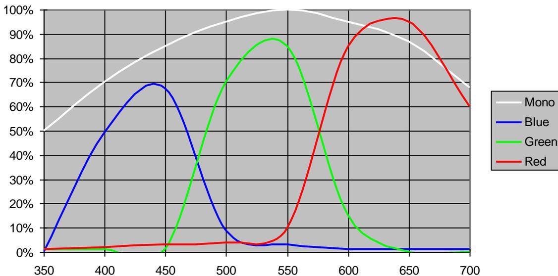
If the image is only scanned with a monochrome sensor this balance cannot be performed. Consequently the gray scale representation of each color depends largely on the response of the CCD chip, the specific color temperature of the illumination system and other factors. The resulting gray scale image will show some colors way too dark and other colors much brighter than present in the original.
